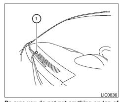
Be sure you do not put anything on top of the autolight sensor (1) located in the top side of the instrument panel. The autolight sensor controls the autolight: if it is covered, the autolight sensor reacts as if it is dark out and the headlights will illuminate. If this occurs while parked with the engine off and the ignition switch placed in the ON position, your vehicle's battery could become discharged.
